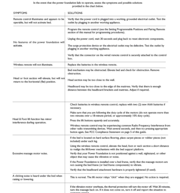
Massage motor overheats or stops. Please notes: Excessive use of the massage motors, over 30 minutes at a time, will cause the motor to shut down and possibly overheat. Extreme care is required when using the massage motors to prevent damage to the motors and/or the adjustable base. Do not use for more than 30 minutes at a time.
